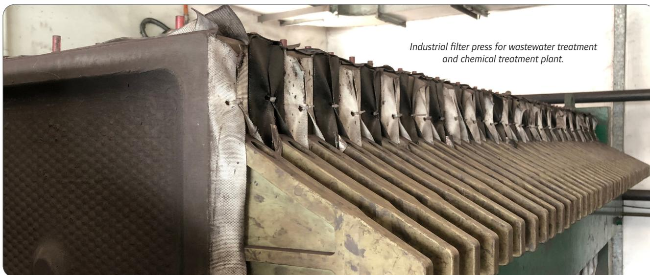
Industrial filter press for wastewater treatment and chemical treatment plant.
